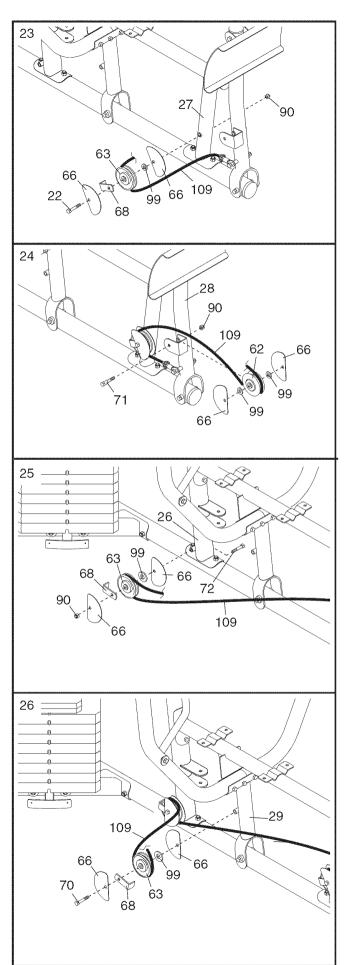
27. Wrap the Press Cable (109) around a "V"-pulley (62). Attach the "V"-pulley, two Half Finger Guards (66), a Large Cable Trap (111), and an M10 Washer (99) inside the bracket on the Left Upright (26) with an M10 x 65mm Bolt (77) and an M10 Nylon Locknut (90). Make sure the Cable Trap and Finger Guards are oriented as shown.
